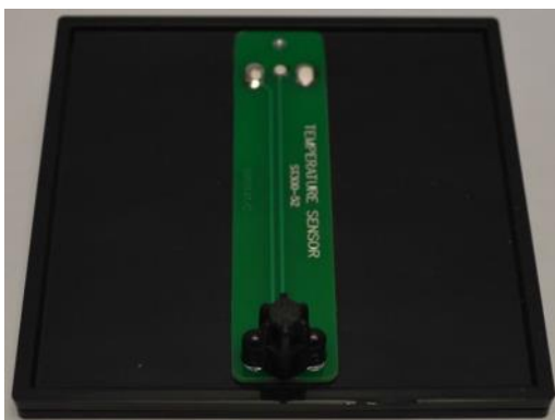
Temperature sensor panel
