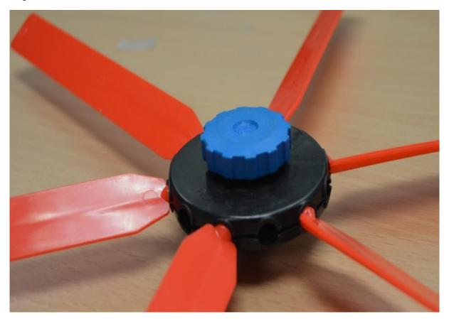
Figure 2: These blades have been set into the hub at the same angle (45<sup>°</sup>)
