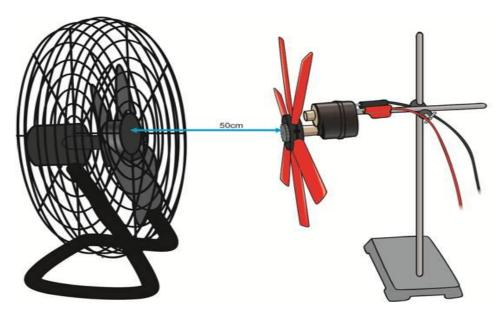
Figure 3: The correct relative positions of the fan and the turbine
