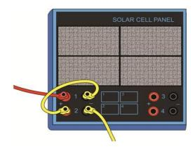
Figure 3: Connecting Cell 1 to Cell 2
