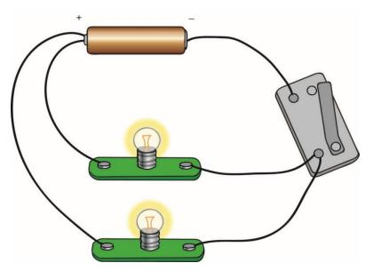
Figure 1: A circuit containing a single battery, a switch and two globes that are in parallel with one another.
