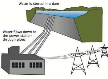
In the power station the water is used to push giant turbines. These in turn cause huge wire coils to spin inside giant magnets, which generates electricity
