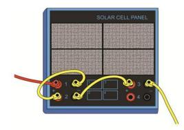
Figure 4: Connecting Cell 2 to Cell 3
