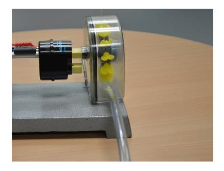
Figure 2. The STELR Pelton wheel that will be used in this activity
