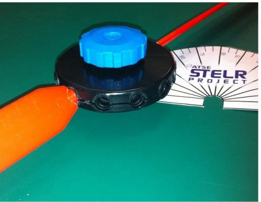
Figure 2: These blades have been set into the hub at the same angle  $(45^{\circ})$
