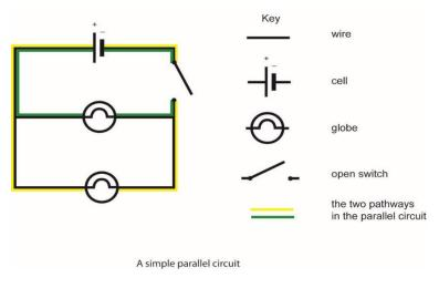
Figure 2: A circuit diagram for a parallel circuit
