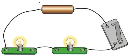
Figure 1: A basic series circuit
