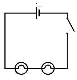
Figure 2: The circuit diagram of the series circuit
