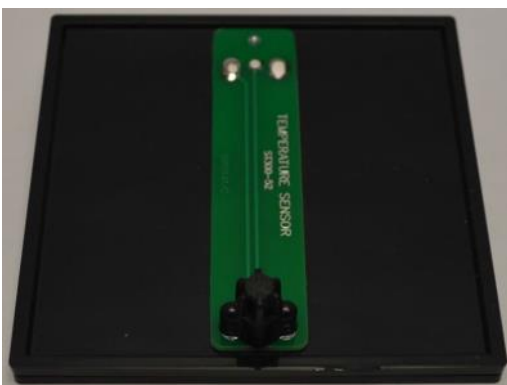
Temperature sensor panel
