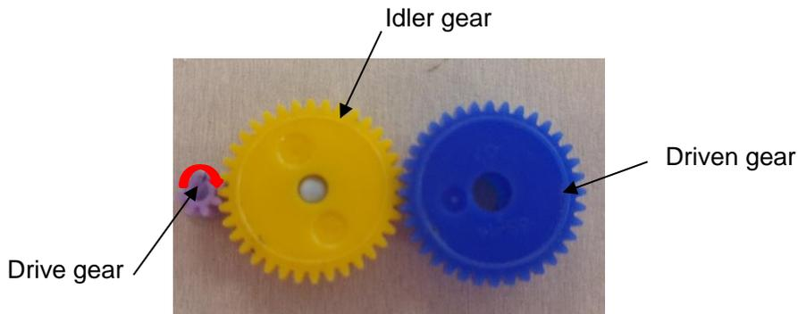
For each gear, write down the direction of rotation (clockwise or anticlockwise).
