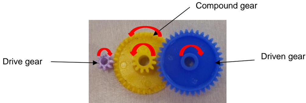
To calculate the gear ratio of a compound gear, multiply the gear ratios of each stage of the gear train.
