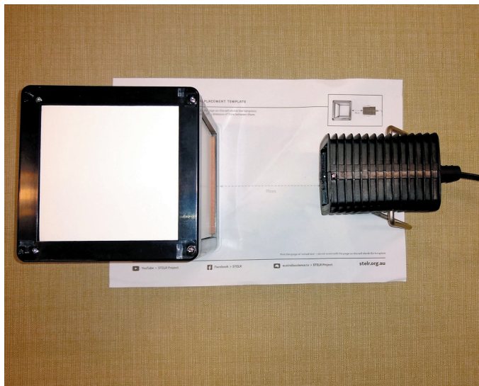
Set up of the equipment showing how to place the lamp on the template
